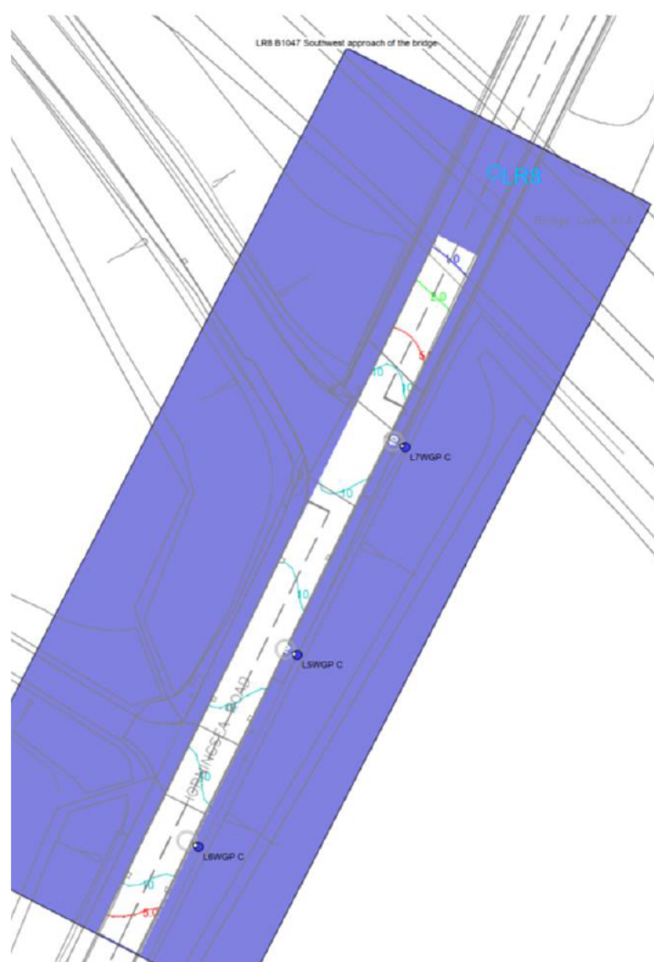
Figure 5.5: LR8 street lighting provision (south west approach to A14 bridge)
